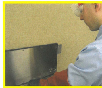
3. ALWAYS wear gauntlets and goggles at all times when using the Decarbonizer
