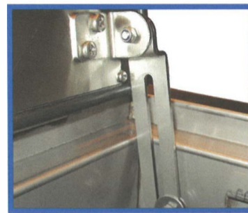
2. Ensure stay arm is in lock position before loading the Decarbonizer
