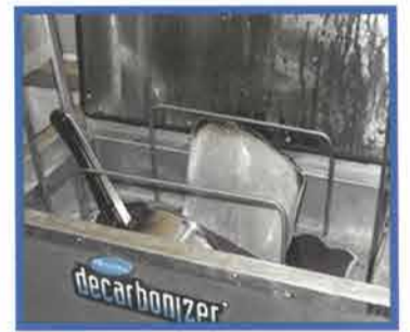
4. Light items - raise, load and lower the basket, ensuring it is fully submerged
