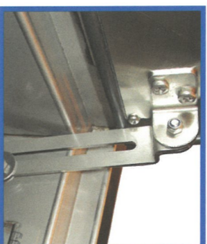
2. Ensure stay arm is in lock position before loading the Decarbonizer
