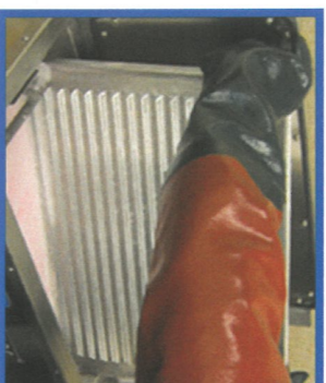
3. Gently immerse grill plates into the Decarbonizer by hand
