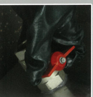
Turn the Red Lever to close Drain Valve and remove Drainage Hose.
