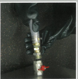
Connect the Drainage Hose to the Drain Valve, turning clockwise to lock in position.
