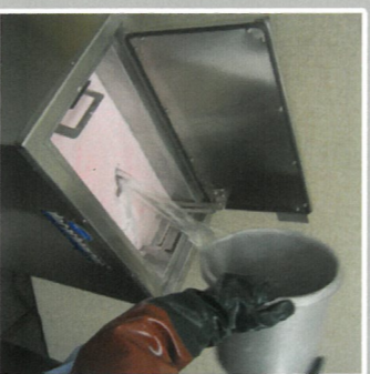
Keep the tank topped up to maximum level. Do not overflow.
