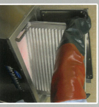
To load larger items, gently immerse by hand whilst the basket is down.
