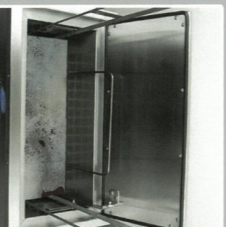
To load the Decarbonizer, secure the basket at the required height.
