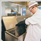
Gently immerse grill plates into the Decarbonizer by hand
