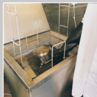
Light Items - raise, load and lower the basket, ensuring it is fully submerged
